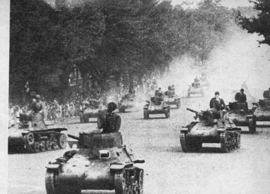
Parade of 2597 armored cars in Tokyo shows sloping face of hull, cylindrical turret with dome-shaped cover and rectangular gun mantlet. Tank weighs about four tons, accommodates two in cramped style.
